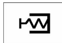
Fig. 26: "Closing spring not charged" indication
